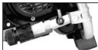
water supply closed (valve lever across)
