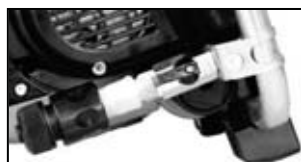
water supply opened (valve lever parallel)
